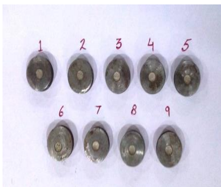
Figure 4.5: EN-31machined work- pieces
