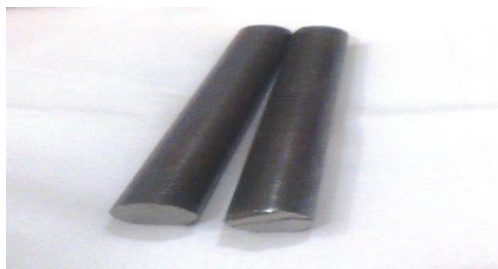
Figure 4.4:work-pieceBars of EN-31
