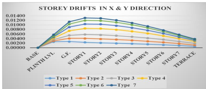
Fig. 9: G+7 Symmetric models Story Drift Graph in X & Y direction
