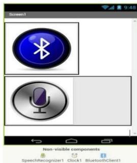
Here the app will implement the function for recognizing the speech along with the Bluetooth client and Clock function. A Google Speech recognizer will get activated when the speak button is clicked. Whatever spoken can be seen in the label "What do you speak" and that is sent to Arduino. The arduino will do the remaining processing works.
