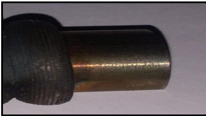
Figure No 14 -Actual Heat Affected Zone 10 mm bar
