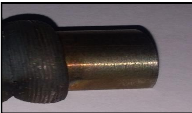
Figure No 10- Actual Heat Affected Zone 14 mm bar
