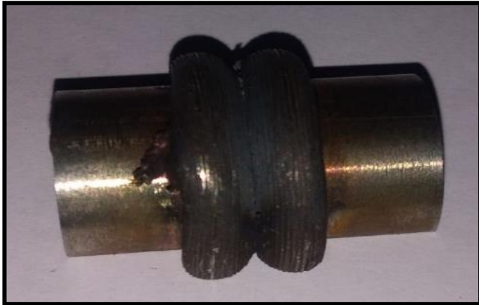
Figure No12- Friction Welded 10mm Bar
