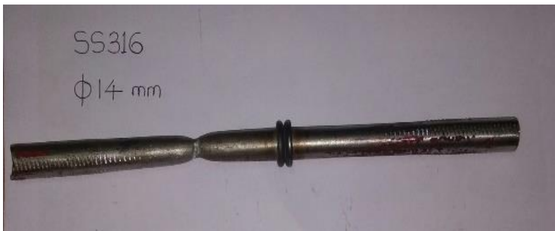
Figure No 16-SS316 14mm Tensile Test Sample
