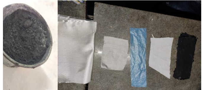
Fig -2: Graphite powder + E glass fibre + Teflon + Perforator + Breather = Composite
