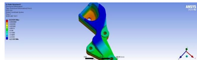
Figure - 33: Directional Deformation of Model 1
