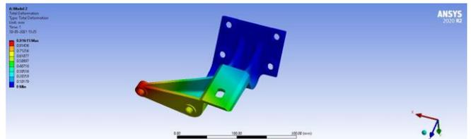
Figure - 14: Total Deformation of Model 2
