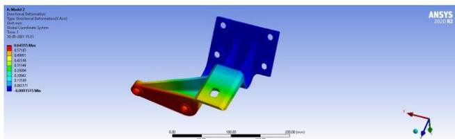
Figure - 22: Directional Deformation of Model 2
