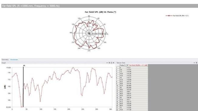
Figure - 60: Far Field SPL vs. Theta for Model 1
