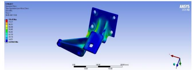
Figure - 24: Equivalent Stress for Model 2
