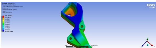
Figure - 21: Directional Deformation of Model 1
