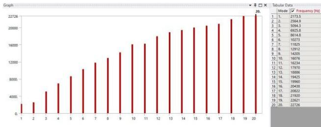
Figure - 75: Mode vs. Frequency for Model 1
