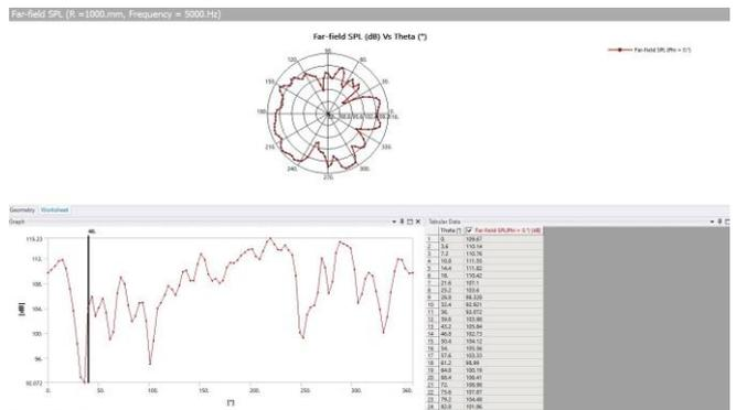
Figure - 46: Far Field SPL vs. Theta for Model 1
