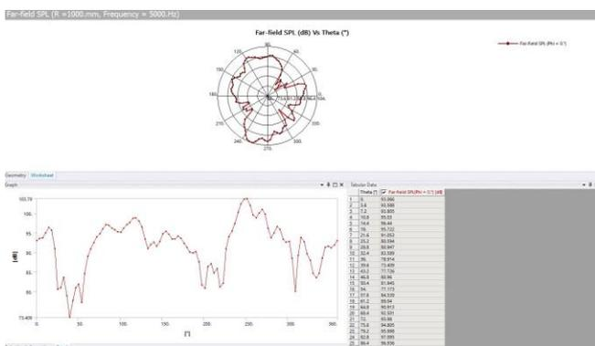
Figure - 88: Far Field SPL vs. Theta for Model 1
