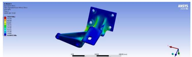
Figure 36: Equivalent Stress for Model 2
