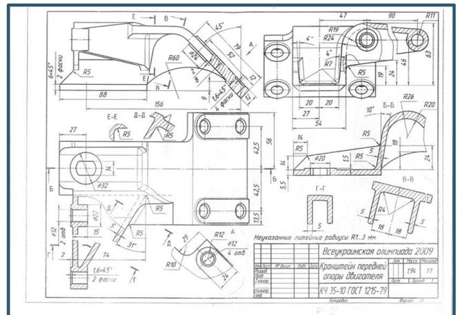
Figure - 4<sup>[7]</sup>: Dimensions Sheet Engine Mount Bracket
