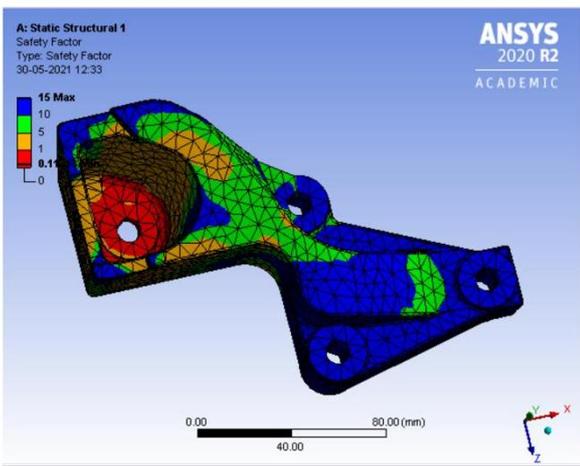
Figure - 93: Fatigue Analysis - Safety Factor
