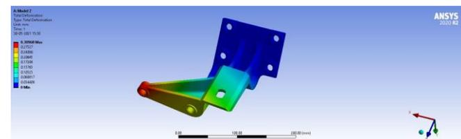
Figure - 34: Directional Deformation of Model 2
