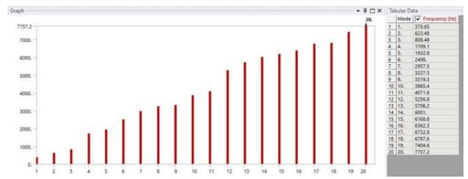
Figure- 90: Mode vs. Frequency for Model 2
