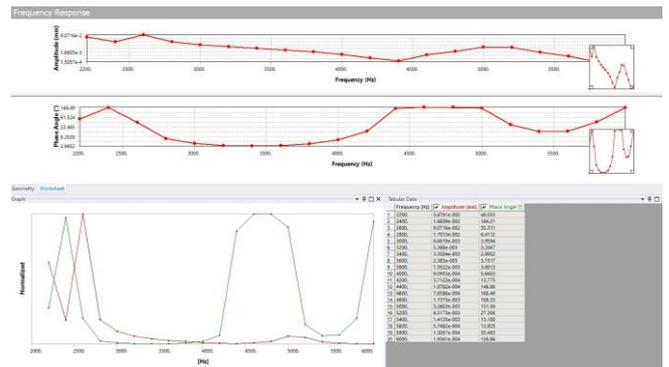
Figure - 71: Frequency Response of Model 1
