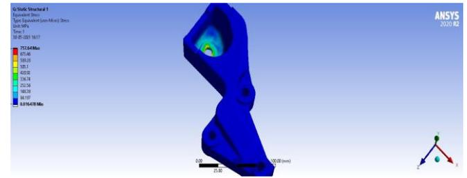
Figure - 23: Equivalent Stress for Model 1
