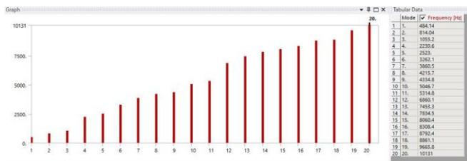
Figure - 78: Mode vs. Frequency for Model 2
