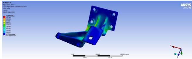
Figure - 18: Equivalent Stress for Model 2
