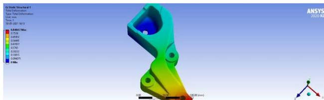
Figure - 31: Total deformation of Model 1
