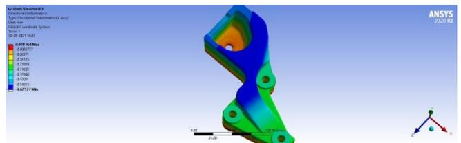
Figure - 15: Directional Deformation of Model 1
