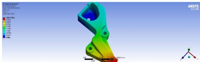
Figure - 19: Total deformation of Model 1
