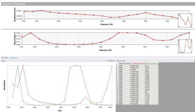
Figure - 41: Frequency Distribution of Model 1
