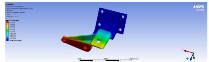
Figure - 28: Directional Deformation of Model 2
