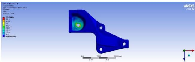
Figure - 29: Equivalent Stress for Model 1
