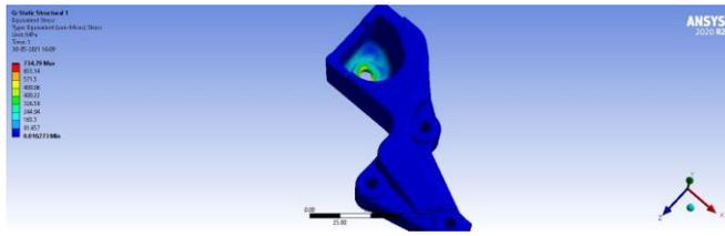
Figure - 17: Equivalent Stress for Model 1
