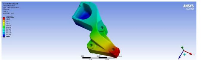
Figure - 25: Total deformation of Model 1
