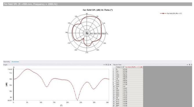
Figure - 91: Far Field SPL vs. Theta for Model 2
