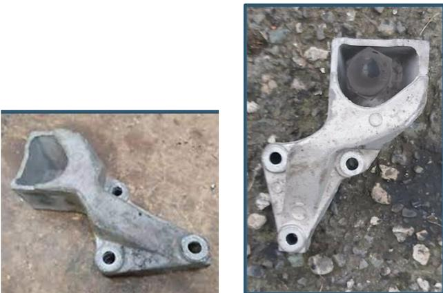
Figure - 2: PEUGEOT 206 GTI 180 Engine Mount Bracket
