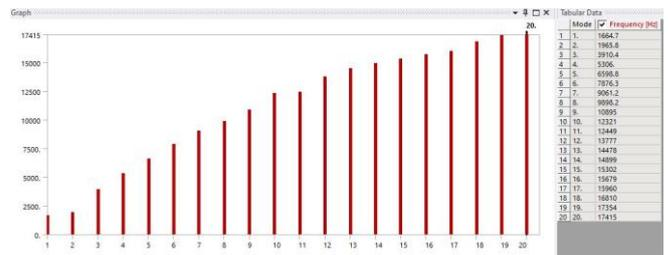
Figure - 89: Mode vs. Frequency for Model 1
