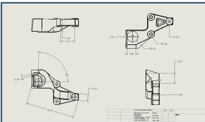
Figure- 3: PEUGEOT 206 GTI 180 Engine Mount Bracket Dimensions Sheet
