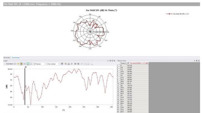
Figure - 74: Far Field SPL vs. Theta for Model 1
