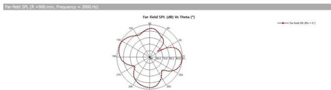
Figure - 77: Far Field SPL vs. Theta for Model 2
