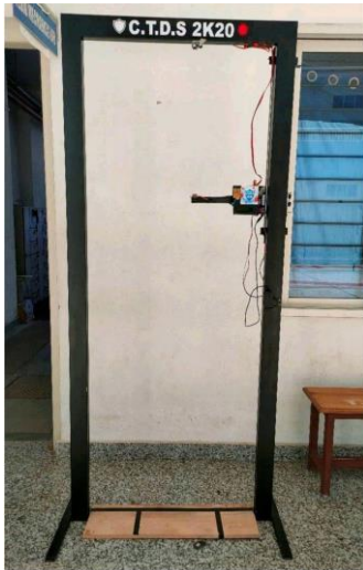
Fig 3: Temperature measurement unit
