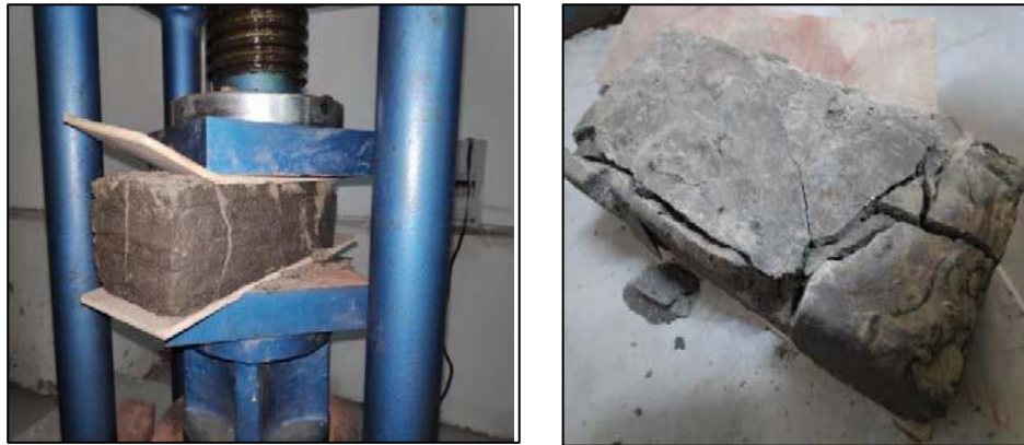
Fig 4: load carrying capacity of Brick under compression test
