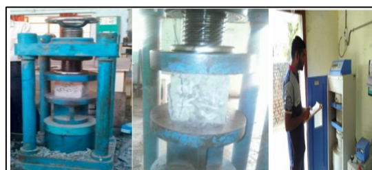
Figure 3: Specimen testing for the brick under compression
