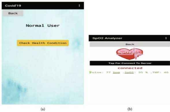
Fig – 10 : a) Normal user Interface b) Measured pulse rate, temperature and oxygen level
