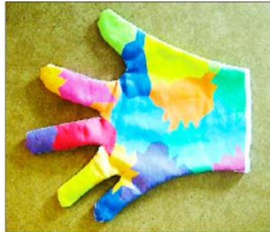
Fig - 6: Colour marker based hand gesture recognition.
