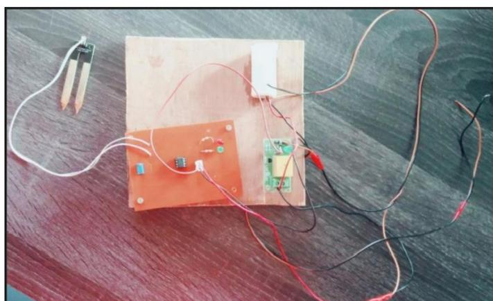
The above shown figures are the working models of the automatic plant watering system.
