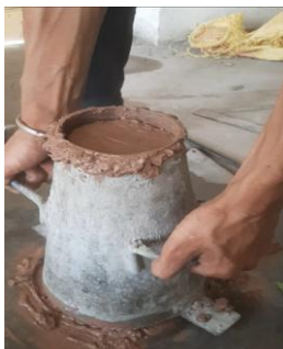
Fig-5: Slump cone
