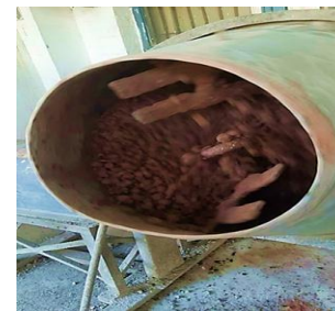
Figure 4.2: Wet mixing in electrically operated drum mixer
