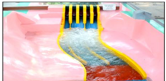
Flow conditions downstream of spillway for Q = 2,875 m 3 /s (Gated flow)
