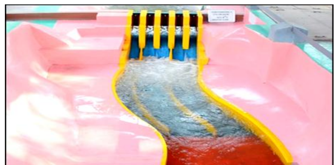
Flow conditions downstream of spillway for Q = 2,875 m 3 /s (Ungated flow)
