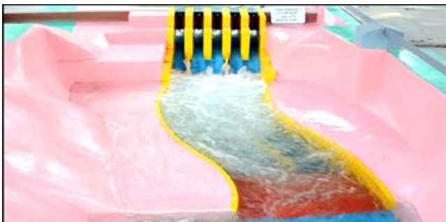
Flow conditions downstream of spillway for Q = 6,900\text{m}^3/\text{s} (Ungated flow)
