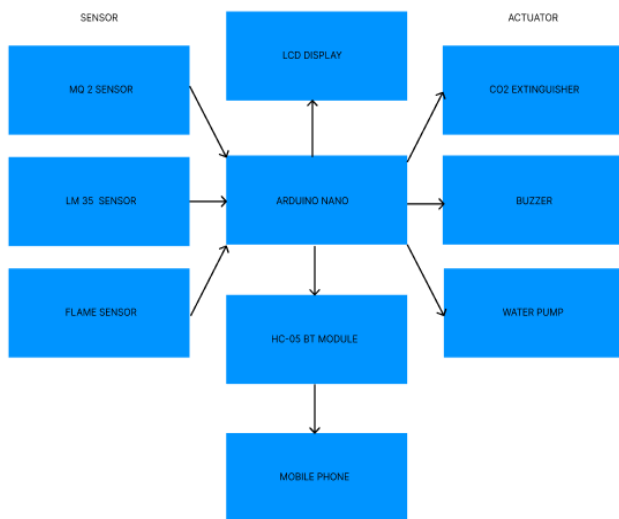
Fig -1: Block Diagram including all essential parts of the fire detection and protection system.
