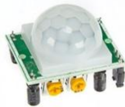
Fig – 4.4: PIR motion sensor
