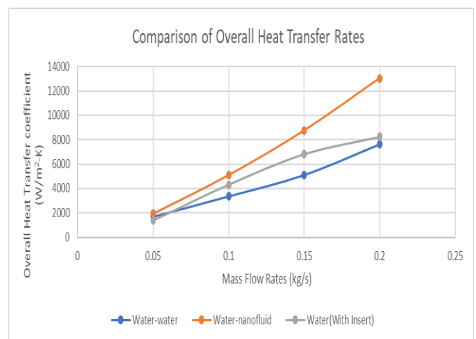
Fig 12 Overall Heat transfer coefficient versus mass flow rate of Cold Fluid in Counter Flow arrangement
