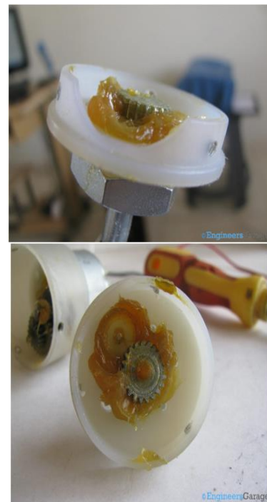
Figure 12: Gear Structure of DC motor
