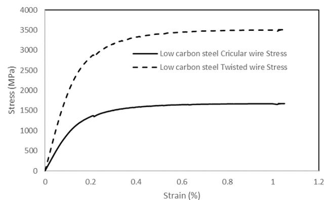
Figure 9: Stress-strain plot of low carbon steel circular wire and twisted wire stress
