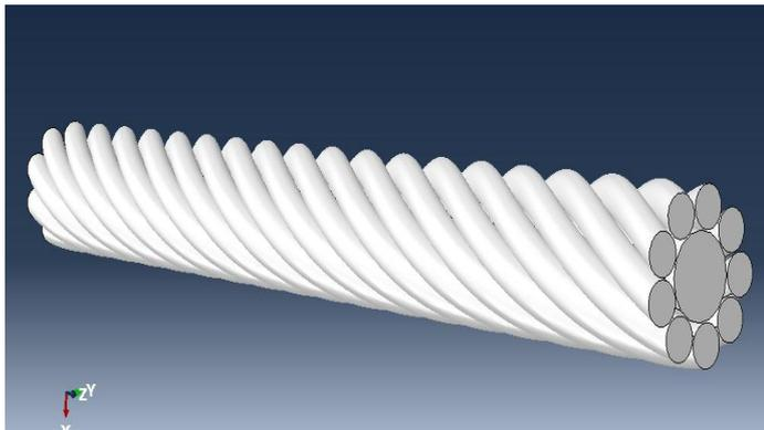
**Figure 1 :** An image of a twisted cable used for FEM simulations
