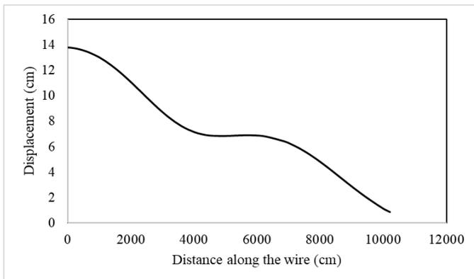
Figure 6: Displacement of twisted wire as a function of its distance
