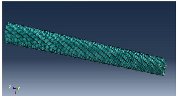
**Figure 4:** Model with 3D meshing and C3D8R (An 8-node linear brick, reduced integration, hourglass control) element type
