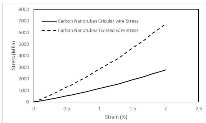
**Figure 11:** Stress-strain curve for the carbon nanotubes for the case of circular and twisted wire stress
