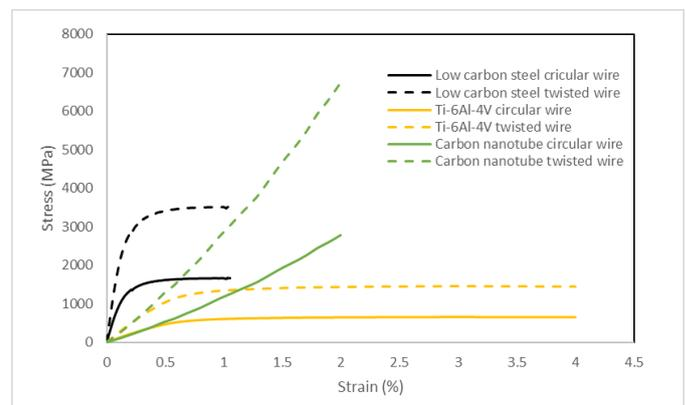
**Figure 12:** Stress-strain curve for the case of circular and twisted wire stress for all the choices of material
