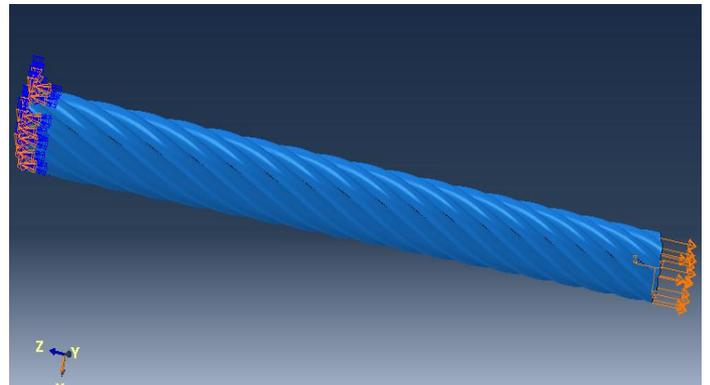
**Figure 3:** Model with fix boundary condition on left side and axial loading along the length (right side) of the wire for FEM simulations
