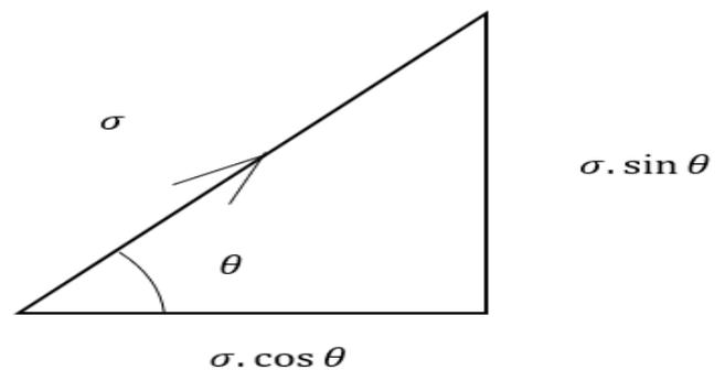
The cos component will become compressive and therefore, compressive forces will act over whole central section which is helical in shape.
