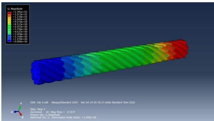
Figure 5: Displacement of the twisted rope
