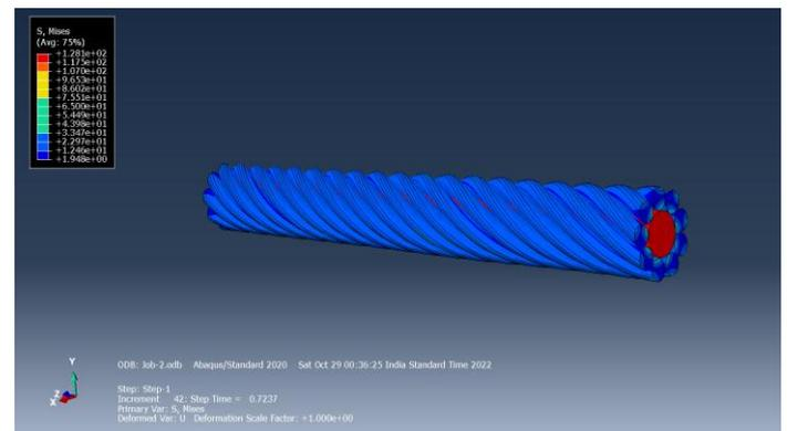
Figure 7: Von mises stresses of the twisted rope
