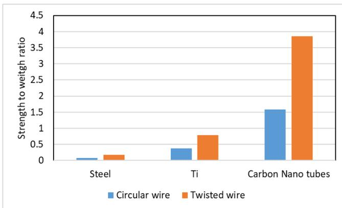
**Figure 13:** Strength to weight ratio of circular and twisted wire for steel, Ti alloy and carbon nanotube
