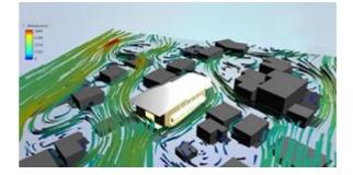
Figure 33 Wind flow analysis around the South façade (Source: Author generated)
