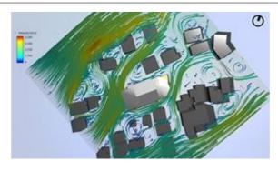
Figure 32 Wind flow analysis – Plan (Source: Author generated)
