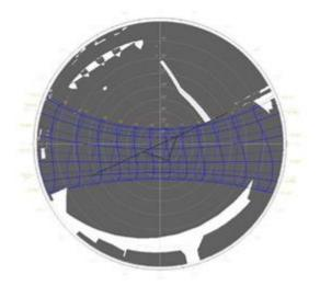
Figure 26 Stereographic diagram of solar shading of a window on South façade (Source: Author generated)
