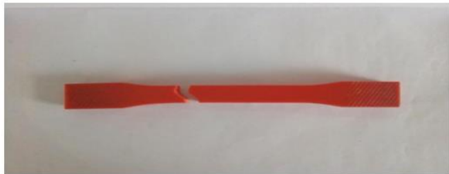
FIG NO-02: TENSILE SPECIMEN OF PLA AFTER THE TEST
