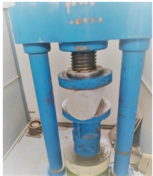
Fig 4.5 Split tensile strength test of cylinders
