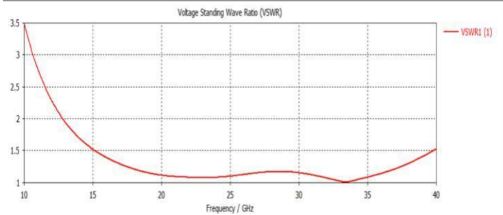
Fig -3: VSWR plot for 5G microstrip patch antenna
