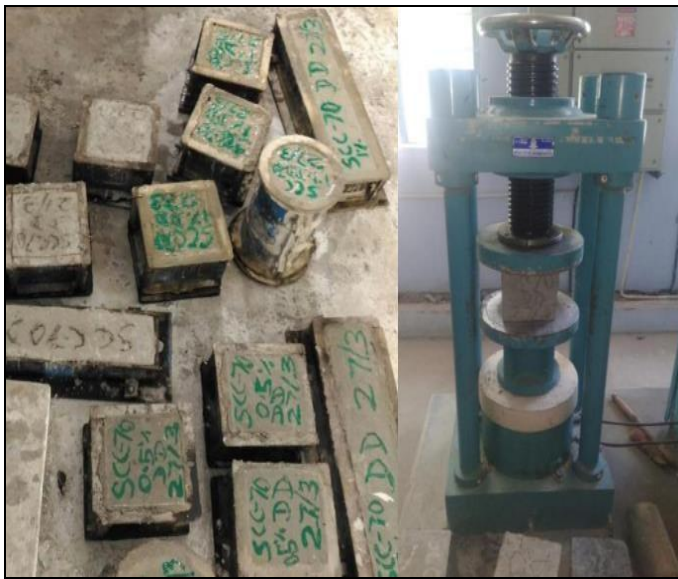
Fig -4: casting and testing of concrete
