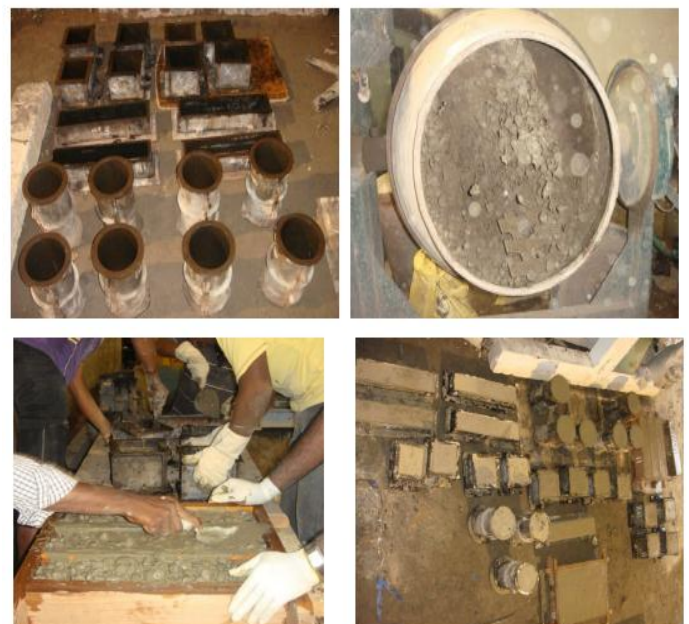
Figure-1: for Casting, Mixing of SFRC, Placing of Concrete, Cast Specimens
