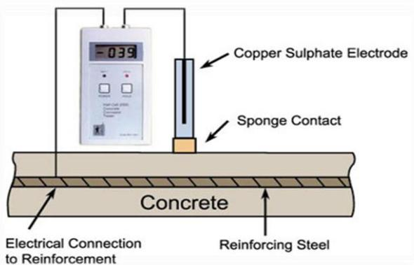
With time chlorides and CO<sub>2</sub> penetrate the concrete and break down that protecting layer. CO<sub>2</sub> lowers the pH of the concrete underneath the extent of balance of the passive movie. In presence of oxygen and water, an electrochemical response initiates the manner of corrosion.
