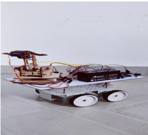
The above given figure shows a smart voice controlled pick and place robot which was built or assembled using arduino uno, HC05 bluetooth module and fitted within a robotic arm for purpose of pick and place. It also shows a four wheel drive chassis whose speed is controlled using the motor drive.
