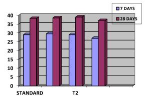
Total 30 cubes were examined for all proportions. 6 cubes were casted for standard proportions. For Each proportion 3 cubes were casted for following 7 and 28 days. Each cube were cured in water tank for respective days and dried for 2 hrs after taking out from tank. Test is carried out.
