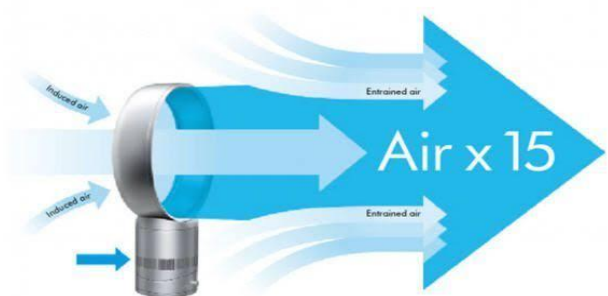
Fig. 2 :- Air Multiplying System
