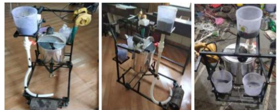
Figure 1: pothole filling machine using waste in mixes
