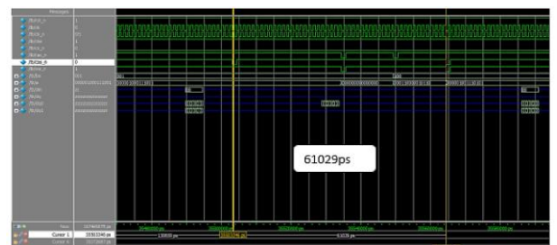
Fig-21: Minimum time between read and write operation in DDR3.
