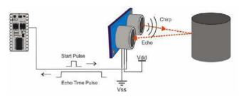
Fig. 2 Ultrasonic Sensor Working
