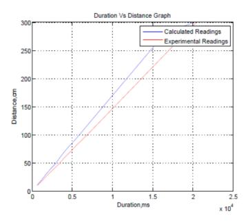
Fig. 7 Response of the Ultrasonic Sensor with Respect to the Obstacle Detection at Various Distances
