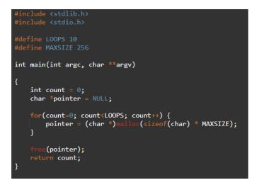
In this example, there are 10 allocations of size MAXSIZE. Every allocation, except for the last, is lost. If no pointer is pointed to the allocated block, it is unrecoverable during program execution. A simple fix to this trivial example is to place the free() call inside of the "for" loop.
