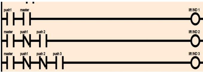
Figure 7 Ladder program for lift indicator
