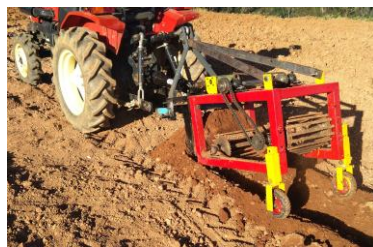
Fig -6: Potato harvesting machine under field testing at ICAR-CPRS, Ooty
