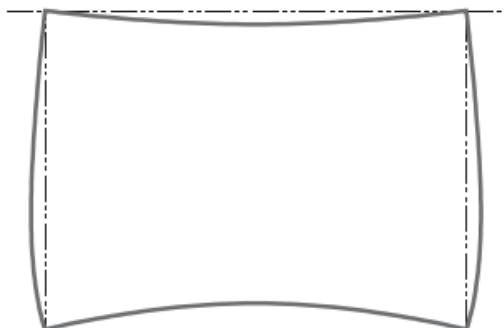
Fig -13: Gravity/Buoyancy deformation pattern of pontoon (Subrata k. Chakrabarti)
