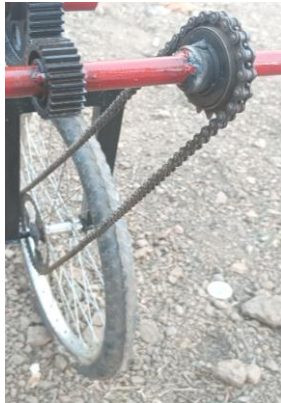
Figure 6 Chain Drive for Power Transmission
