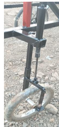
Figure 5 Suspensions connected to Frame and Wheels.
