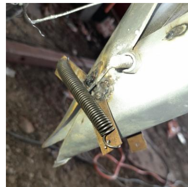
Figure 9 Tension Spring for Opening/Closing
