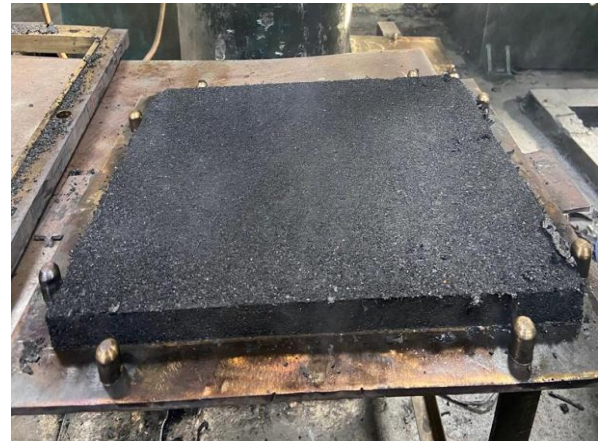
Figure 2-b: The Rubber-Resin tiles sheet during removal from the plate
