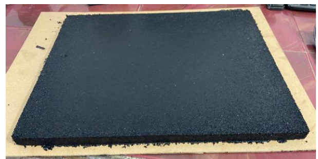
Figure 4: Compressed Rubber Resin Tiles Sheet After Dry Out
