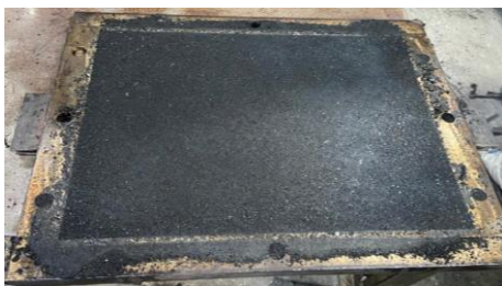
Figure 2-a: The Rubber-Resin tiles sheet immediately after pressing
