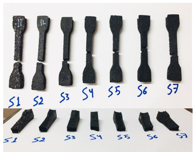
Figure 6: Fracture after tensile stress.
