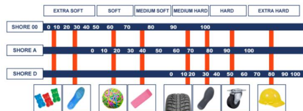
Figure 7: Hardness values range per application
