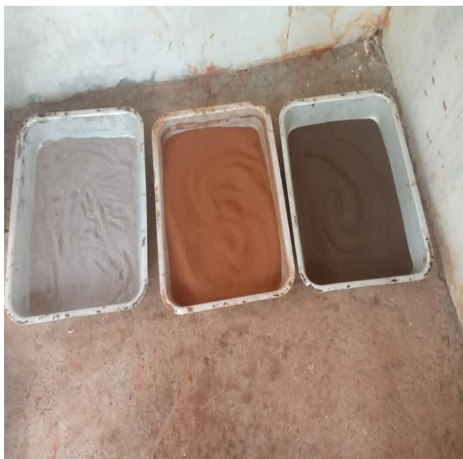
Fig -2: Sieved Boiler Ash, Soil and Sludge
