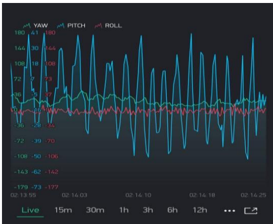
Fig. 6: Change in Values of Pitch, Yaw, and Roll when the system is placed in a water body
