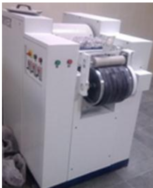
Figure 1: Lab model carding machine
