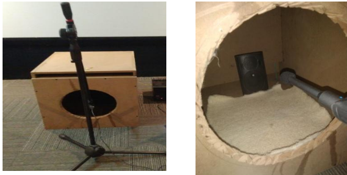
Figure-3 Experimental setup for measuring sound absorption by reverberation time method
