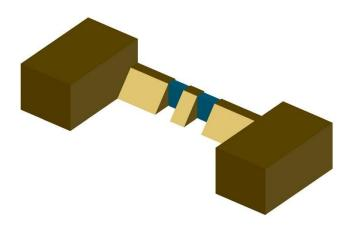
In pemanal, the existing check dam has inefficiency in its purpose due to deterioration and lack of proper working structure. During rainy season when the water overflows the solid waste gets accumulated in the checkdam resulting in poor functioning of its designed purpose. Based on our survey we had designed a model to reconstruct the checkdam considering the site. The figure shows the 3D view of model being designed for reconstruction. It has a width of 5m and a height of 1.5m.
