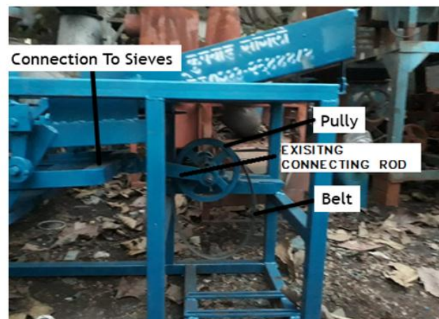
Fig -1: Existing Sorting Platform
