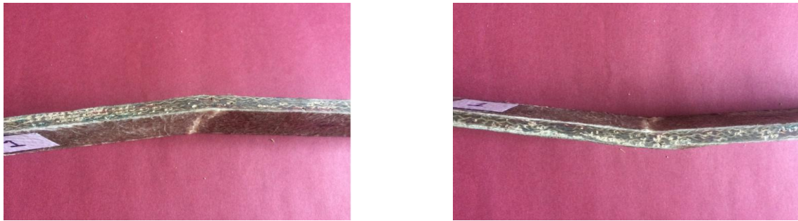
Fig.19. (a) and (b) shows Images of flexural fractured specimen of sample 1
