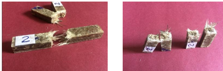
Fig.23. (a) and (b) show Images of impact fractured specimen of sample 2.
