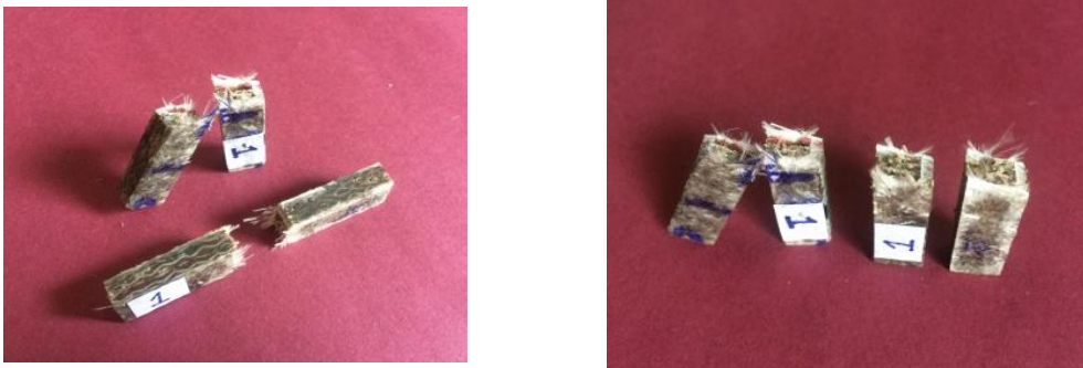
Fig.22. (a) and (b) show Images of impact fractured specimen of sample 1
