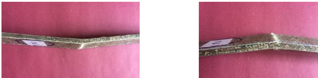
Fig.20. (a) and (b) show Images of flexural fractured specimen of sample 2
