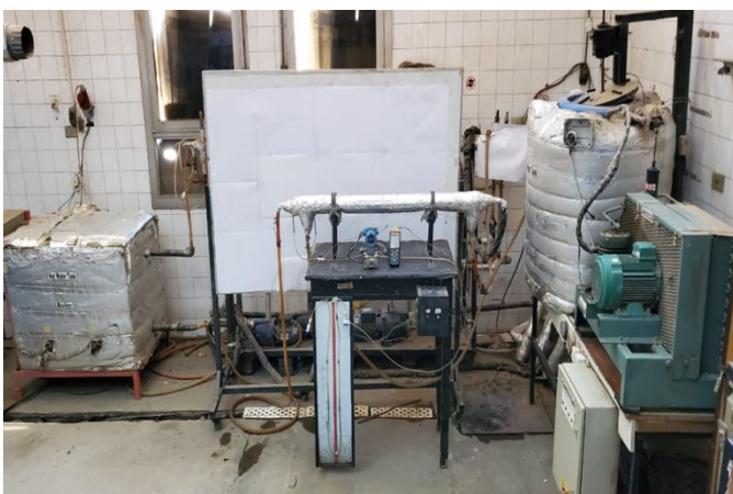
Fig.1 Experimental double tube heat exchanger with instrumentation
