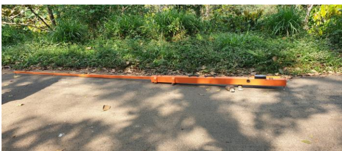
Fig - 3: Benkelman beam placed on location
