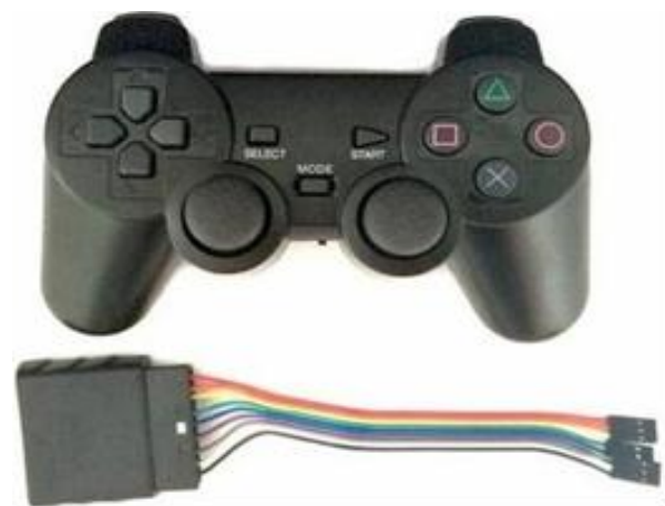
Fig -3: 2.4Ghz RF Controller and receiver
