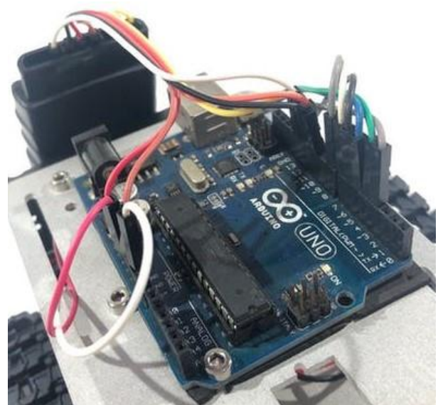
Fig -4: Arduino interfaced with RF Receiver
