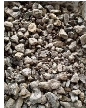
Fig -2: Recycled aggregates containing attached mortar
