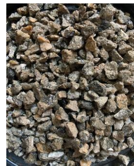
Fig -3: Recycled aggregates devoid of attached mortar after treatment
