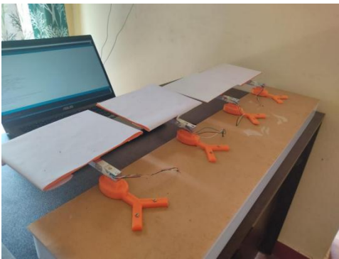
Fig -3: Hardware set- up (base of the cabinet) along with four load cells
