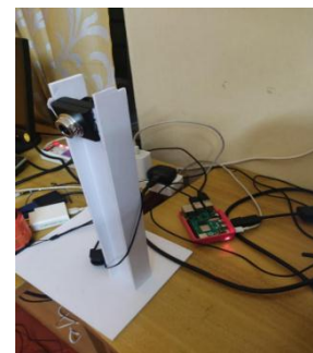
Fig -6: Raspberry Pi image processing setup
