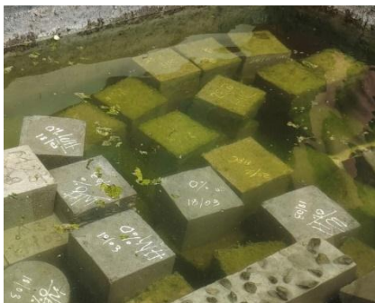
Figure 10 Immersing concrete cubes in water for 48 hours
