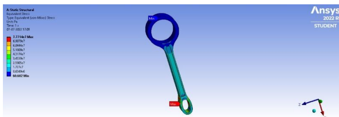
Figure 4: Equivalent Stress of Aluminum alloy Connecting rod
